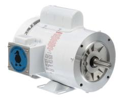
Leeson Washguard White Duck premium efficiency AC induction motor, washdown, 1hp, 1-phase, 115/208-230 VAC, 1800rpm, TEFC, NEMA 56C frame, rolled steel, C-face/rigid base mount.
