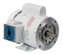
Leeson Washguard White Duck standard efficiency AC induction motor, washdown, 1/2hp, 1-phase, 115/208-230 VAC, 1800rpm, TEFC, NEMA 56C frame, rolled steel, C-face/rigid base mount.
