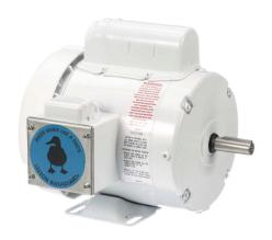
Leeson Washguard White Duck standard efficiency AC induction motor, washdown, 1/2hp, 1-phase, 115/208-230 VAC, 1800rpm, TEFC, NEMA 56 frame, rolled steel, rigid base mount.
