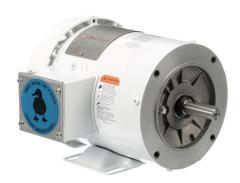
Leeson Washguard White Duck standard efficiency AC induction motor, washdown and inverter rated, 3/4hp, 3-phase, 208-230/460 VAC, 1800rpm, TEFC, 56C frame, rolled steel, C-face/rigid base mount.
