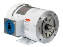
Leeson Washguard White Duck standard efficiency AC induction motor, washdown and inverter rated, 1/2hp, 3-phase, 208-230/460 VAC, 1800rpm, TEFC, NEMA 56C frame, rolled steel, C-face/rigid base mount.
