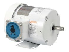
Leeson Washguard White Duck standard efficiency AC induction motor, washdown and inverter rated, 3/4hp, 3-phase, 208-230/460 VAC, 1800rpm, TEFC, 56 frame, rolled steel, rigid base mount.
