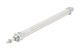
Metal Work pneumatic cylinder, ISO 6432 non-repairable, 25mm bore, 10mm rod diameter, 300mm stroke, double acting, magnetic piston, universal mount.
