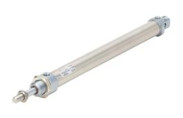
Metal Work pneumatic cylinder, ISO 6432 non-repairable, 25mm bore, 10mm rod diameter, 250mm stroke, double acting, magnetic piston, universal mount.
