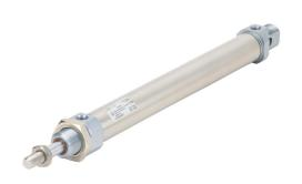
Metal Work pneumatic cylinder, ISO 6432 non-repairable, 25mm bore, 10mm rod diameter, 200mm stroke, double acting, magnetic piston, universal mount.
