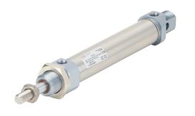
Metal Work pneumatic cylinder, ISO 6432 non-repairable, 25mm bore, 10mm rod diameter, 100mm stroke, double acting, magnetic piston, universal mount.
