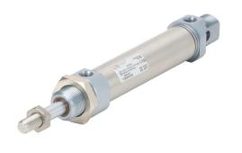
Metal Work pneumatic cylinder, ISO 6432 non-repairable, 25mm bore, 10mm rod diameter, 75mm stroke, double acting, magnetic piston, universal mount.
