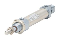
Metal Work pneumatic cylinder, ISO 6432 non-repairable, 25mm bore, 10mm rod diameter, 50mm stroke, double acting, magnetic piston, universal mount.
