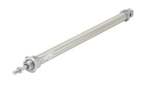
Metal Work pneumatic cylinder, ISO 6432 non-repairable, 20mm bore, 8mm rod diameter, 300mm stroke, double acting, magnetic piston, universal mount.
