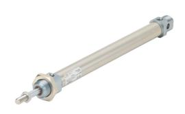
Metal Work pneumatic cylinder, ISO 6432 non-repairable, 20mm bore, 8mm rod diameter, 200mm stroke, double acting, magnetic piston, universal mount.
