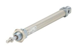
Metal Work pneumatic cylinder, ISO 6432 non-repairable, 20mm bore, 8mm rod diameter, 150mm stroke, double acting, magnetic piston, universal mount.
