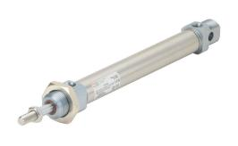
Metal Work pneumatic cylinder, ISO 6432 non-repairable, 20mm bore, 8mm rod diameter, 125mm stroke, double acting, magnetic piston, universal mount.
