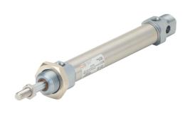
Metal Work pneumatic cylinder, ISO 6432 non-repairable, 20mm bore, 8mm rod diameter, 100mm stroke, double acting, magnetic piston, universal mount.
