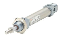
Metal Work pneumatic cylinder, ISO 6432 non-repairable, 20mm bore, 8mm rod diameter, 50mm stroke, double acting, magnetic piston, universal mount.
