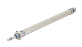
Metal Work pneumatic cylinder, ISO 6432 non-repairable, 16mm bore, 6mm rod diameter, 200mm stroke, double acting, magnetic piston, universal mount.
