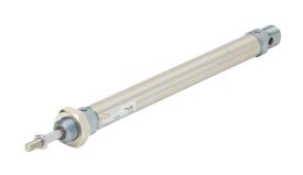
Metal Work pneumatic cylinder, ISO 6432 non-repairable, 16mm bore, 6mm rod diameter, 150mm stroke, double acting, magnetic piston, universal mount.
