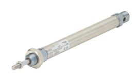
Metal Work pneumatic cylinder, ISO 6432 non-repairable, 16mm bore, 6mm rod diameter, 125mm stroke, double acting, magnetic piston, universal mount.
