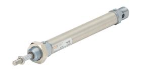
Metal Work pneumatic cylinder, ISO 6432 non-repairable, 16mm bore, 6mm rod diameter, 100mm stroke, double acting, magnetic piston, universal mount.
