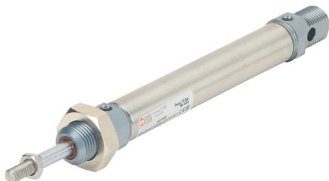
Metal Work pneumatic cylinder, ISO 6432 non-repairable, 16mm bore, 6mm rod diameter, 75mm stroke, double acting, magnetic piston, universal mount.
