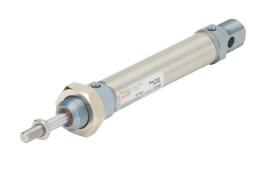
Metal Work pneumatic cylinder, ISO 6432 non-repairable, 16mm bore, 6mm rod diameter, 50mm stroke, double acting, magnetic piston, universal mount.
