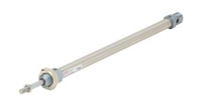
Metal Work pneumatic cylinder, ISO 6432 non-repairable, 12mm bore, 6mm rod diameter, 200mm stroke, double acting, magnetic piston, universal mount.
