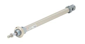
Metal Work pneumatic cylinder, ISO 6432 non-repairable, 12mm bore, 6mm rod diameter, 150mm stroke, double acting, magnetic piston, universal mount.
