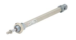
Metal Work pneumatic cylinder, ISO 6432 non-repairable, 12mm bore, 6mm rod diameter, 125mm stroke, double acting, magnetic piston, universal mount.
