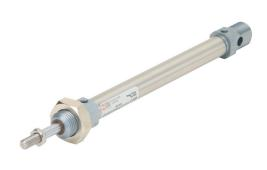
Metal Work pneumatic cylinder, ISO 6432 non-repairable, 12mm bore, 6mm rod diameter, 100mm stroke, double acting, magnetic piston, universal mount.
