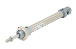
Metal Work pneumatic cylinder, ISO 6432 non-repairable, 12mm bore, 6mm rod diameter, 75mm stroke, double acting, magnetic piston, universal mount.
