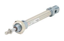
Metal Work pneumatic cylinder, ISO 6432 non-repairable, 12mm bore, 6mm rod diameter, 50mm stroke, double acting, magnetic piston, universal mount.
