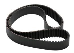
SureMotion timing belt, 8mm 8M pitch, 30mm wide, 140 tooth, 1120mm pitch length (circumference), neoprene, fiberglass reinforced.
