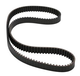
SureMotion timing belt, 8mm 8M pitch, 20mm wide, 140 tooth, 1120mm pitch length (circumference), neoprene, fiberglass reinforced.
