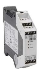
ASO Safety Solutions safety relay, safety mat/edges, 1-channel, 24 VAC/VDC or 120 VAC, (2) N.O. safety output(s), (1) N.O. monitoring output(s), fixed screw terminals.
