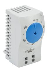
Stego thermostat, adjustable, N.O. (close on rise) 14 to 122 deg F, 12.6 deg F switching differential, 35mm DIN rail mount, for electrical enclosure climate control.
