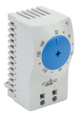
Stego thermostat, adjustable, N.O. (close on rise) 32 to 140 deg F, 12.6 deg F switching differential, 35mm DIN rail mount, for electrical enclosure climate control.
