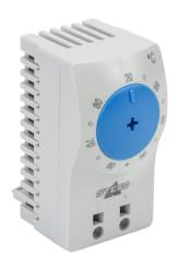
Stego thermostat, adjustable, N.O. (close on rise) 20 to 80 deg C, 7K switching differential, 35mm DIN rail mount, for electrical enclosure climate control.
