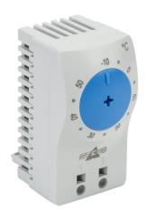
Stego thermostat, adjustable, N.O. (close on rise) -10 to 50 deg C, 7K switching differential, 35mm DIN rail mount, for electrical enclosure climate control.
