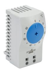
Stego thermostat, adjustable, N.O. (close on rise) 0 to 60 deg C, 7K switching differential, 35mm DIN rail mount, for electrical enclosure climate control.
