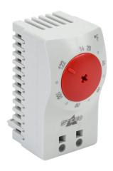
Stego thermostat, adjustable, N.C. (open on rise) 14 to 122 deg F, 12.6 deg F switching differential, 35mm DIN rail mount, for electrical enclosure climate control.
