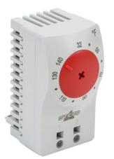
Stego thermostat, adjustable, N.C. (open on rise) 32 to 140 deg F, 12.6 deg F switching differential, 35mm DIN rail mount, for electrical enclosure climate control.
