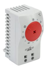
Stego thermostat, adjustable, N.C. (open on rise) 20 to 80 deg C, 7K switching differential, 35mm DIN rail mount, for electrical enclosure climate control.
