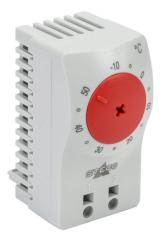
Stego thermostat, adjustable, N.C. (open on rise) -10 to 50 deg C, 7K switching differential, 35mm DIN rail mount, for electrical enclosure climate control.
