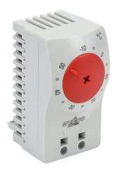
Stego thermostat, adjustable, N.C. (open on rise) -10 to 50 deg C, 7K switching differential, 35mm DIN rail mount, for electrical enclosure climate control.
