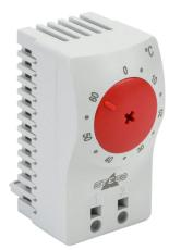
Stego thermostat, adjustable, N.C. (open on rise) 0 to 60 deg C, 7K switching differential, 35mm DIN rail mount, for electrical enclosure climate control.
