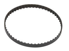
SureMotion timing belt, 1/5in XL pitch, 1/4in wide, 55 tooth, 11in pitch length (circumference), neoprene, fiberglass reinforced.
