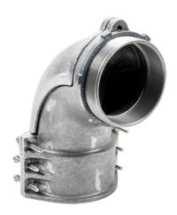
Halex fitting, zinc die cast, 90-degree, 3-1/2in trade size, screw clamp conduit connection. Package of 1. For use with flexible metal conduit (FMC). Screws and locknut included.
