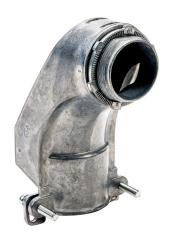
Halex fitting, zinc die cast, 90-degree, 1-1/2in trade size, screw clamp conduit connection. Package of 5. For use with flexible metal conduit (FMC). Screws and locknut included.
