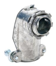
Halex fitting, zinc die cast, 90-degree, 1/2in trade size, screw clamp conduit connection. Package of 25. For use with flexible metal conduit (FMC), AC cable (BX), MC cable. Screws and locknut included.
