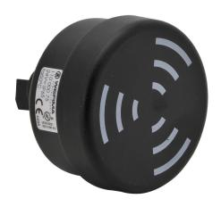
WERMA audible alarm buzzer, 100 dB at 1m, 1.6 kHz to 3.4 kHz tone frequency, (8) selectable tone(s), 24 VAC/VDC, 22mm, panel mount, ABS/polycarbonate housing, black, IP65.
