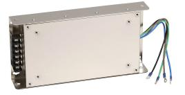
AutomationDirect EMI input filter, 230 VAC, 3-phase, 10A, panel mount, EMI/RFI filtering, drive rated, standard performance, screw terminals and ring terminals. For use with 3-phase AC drives.
