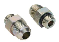
HY-TECH hydraulic fluid adapter, straight, plated steel body, (1) -10 male JIC 37 deg and (1) -8 male o-ring boss. Package of 2.
